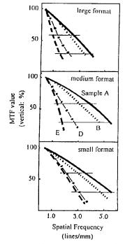
Figure 4. MTF Characteristics of sample prints.
